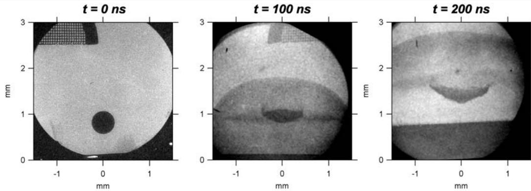
**Fig. 3** Pre-shot radiograph ( $t = 0$  ns) and experimental radiographs at  $t = 100$  and  $200$  ns. The initial position ( $\mu\text{m}$ ) of the ball ( $r, z$ ) is (208, 1229), (160, 1114) and (166, 1195) respectively. The nominal position of the ball is (0, 1050) where  $r = 0$  corresponds to a position
