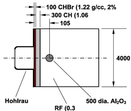
**Fig. 2** The target design for the shock-sphere interaction experiment. All dimensions are in  $\mu\text{m}$ . The hohlraum measures 1.6 mm in diameter and is 1.2 mm long and the foam cylinder measure 4000  $\mu\text{m}$  in length
